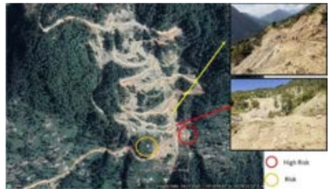
Figure 6: Google image of Dhairing showing landslide and settlements in risk and high risk.
