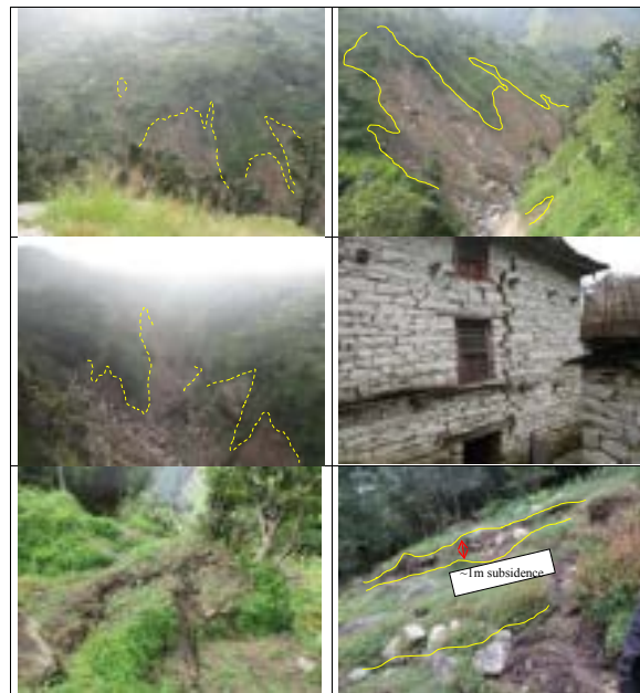
Figure 20: a), b) c) landslides at the downhill slope of the Alleri Gaun; d) crack on house since landslide event and e) cultivated land above landslide; f) complex failure on colluvium above Alleri village.
