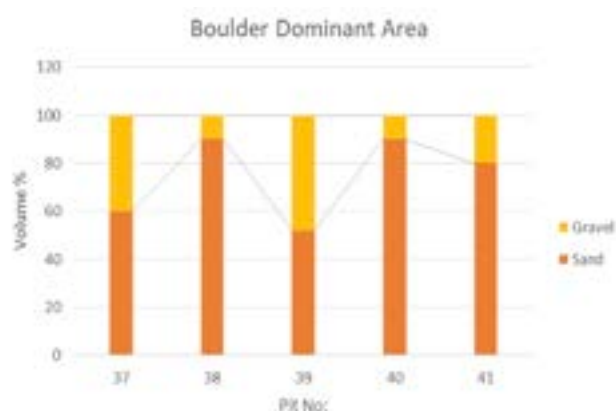
Figure 3: Calculated volumetric percentage of sand or gravel for pits 37-41 representing Boulder Dominant area.
