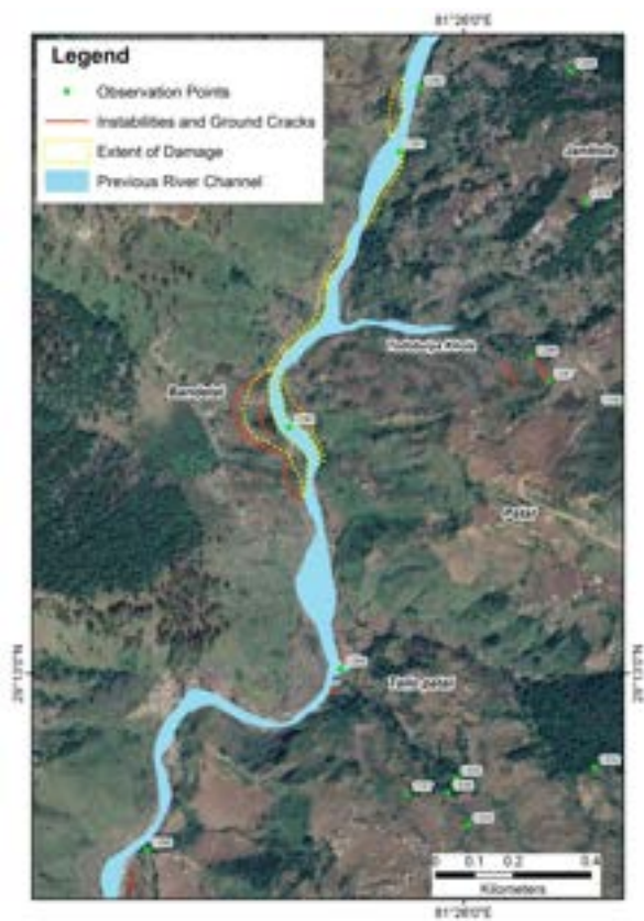
Figure 14: Satellite image of the Patal-Bandatal area showing instabilities and the observation points.
