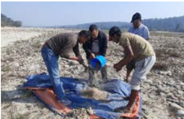
Plate 4: Wire mesh is used to separate the gravel from sand
