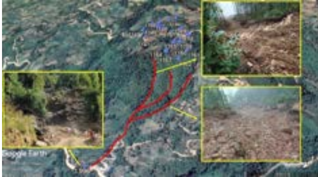
Figure 13: Three limbs of Churi surface slide that killed a child in Sirsuwa (Mudkuwa)
