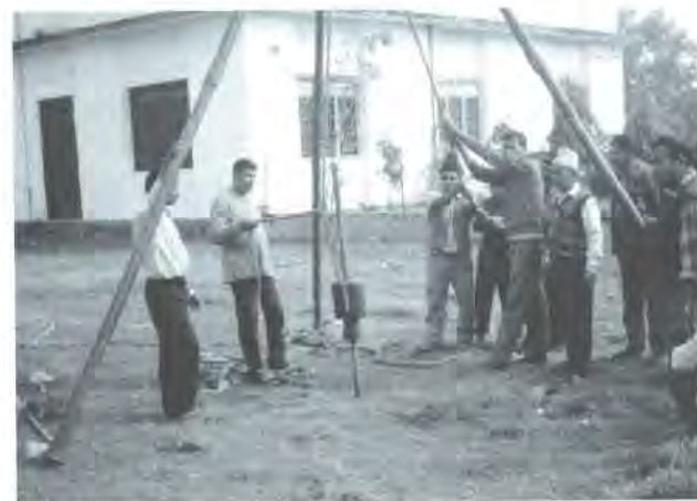
Fig. 3. Men Performing Standard Penetration Test (SPT) in the field.
