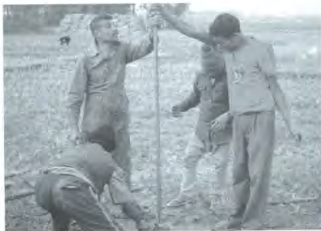
Fig. 2. Men performing Auger hole drill in the field
