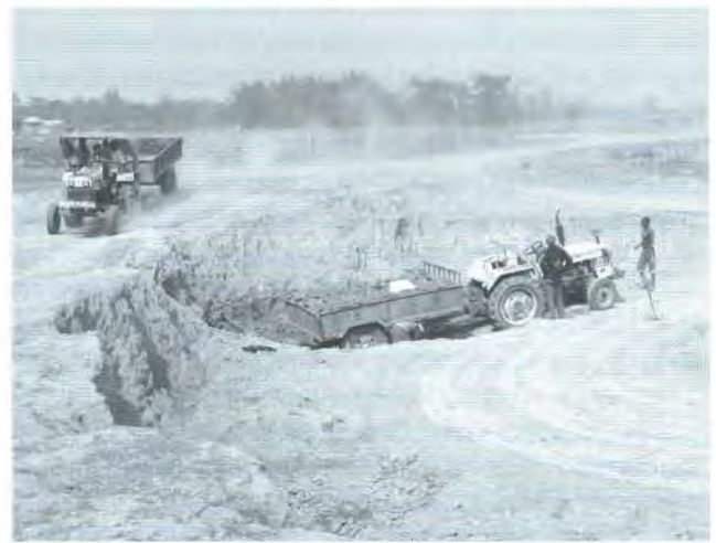
Fig. 11. Improper clay mining from the right bank of Singhiya Khola near Bhatigachh.
