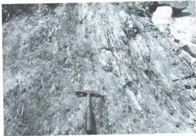
Fig. 3: Grey phyllite and grey to white sericitic quartzites of Dubbidanda Formation in Khadam Khola
