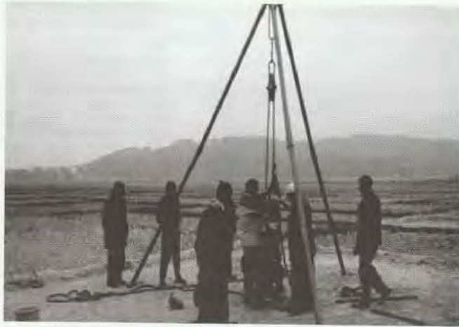
Photo 1 Field personnel preparing for Standard Penetration Test
