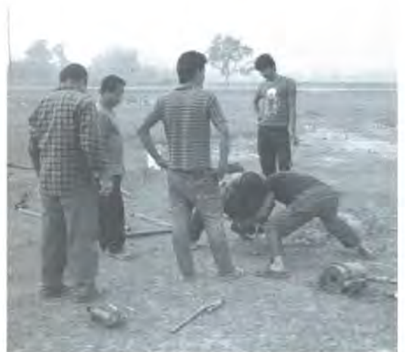
Fig. 3: Samples being recovered by auguring
