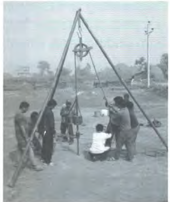
Fig. 2: Field personnel performing SPT
