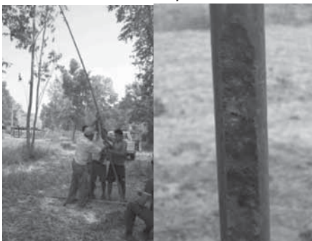
Fig. 2: Field personnel performing SPT and Samples being recovered by auguring.
