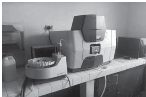
Fig. 2: ED-XRF and AAS in the Conventional Lab for metallic ore analysis in DMG
