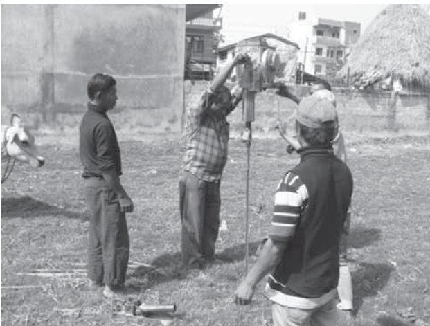
Fig. 5: Performing power auger test
