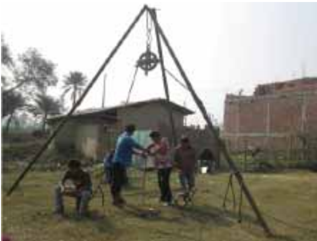
SPT for Engineering and Environmental Geological Mapping of Jaleswor Municipality, Mahottari
