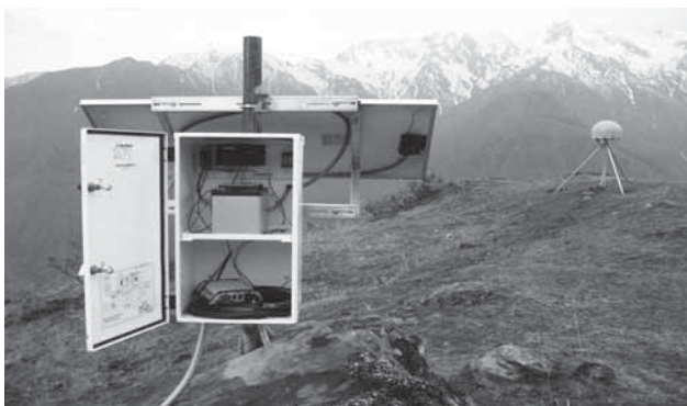
Fig. 9: Photograph of Global Positioning System (GPS) station in Humla.
