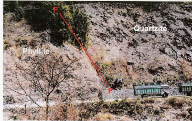
Photo 12: Vegetation including trees grown along the fault contact between Phyllite and Quartzite at Armadi.
